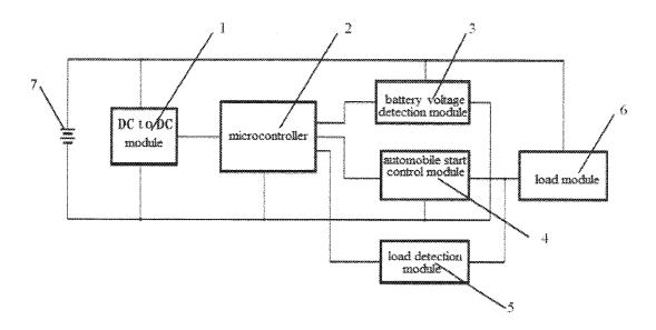
Figure 1 is a block diagram showing one embodiment of an automobile charger that includes DC to DC module 1, microcontroller 2, battery voltage detection module 3, automobile start control module 4, load detection module 5, load module 6, and direct current power supply 7 (the
