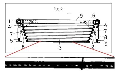
Annotated Song's Figure 2 from page 25 of the Petition depicting water tank 3 with extended support legs 7. According to Patent Owner, the bottom area of water tank 3 does not depict a consistent pattern of cross-hatching or markings. Prelim. Resp. 25. Patent Owner also observes that Song describes the entirety of lid 9 as having a rigid material, but does not show cross-hatching in lid body 9. *Id.* at 27.
