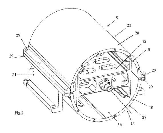
Figure 2 is a perspective view of a rotor and housing of a centrifuge with its front side wall removed. Ex. 1001, 9:30–31.
