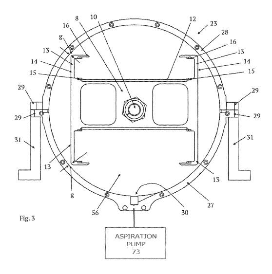
Figure 3 is a front view of a rotor and housing of a centrifuge with its front side wall removed. Ex. 1001, 9:33–34.
