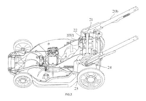
Figures 1 and 2 depict schematic views of an exemplary garden tool, lawnmower 100. Ex. 1001, 1:66–2:1. Mower 100 includes main body 10 and handle 20, which is rotatably connected to main body 10. *Id.* at 2:34–36. The end of handle 20 closest to the user includes an operation assembly, which includes trigger B. *Id.* at 2:49–56.
