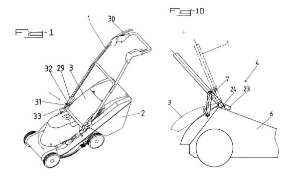
Figure 1 depicts "a perspective view of a mower," and Figure 10 depicts a "partial schematic view[] showing [an] embodiment[] of the cutting-blade activation means" for a mower. Ex. 1014, 3:5–6, 3:22–23. Outils's lawnmower includes handlebar 1, cut-grass receiving receptacle 2, and safety cover 3. *Id.* at 3:35–4:3. In the embodiment of Figure 10, link 7 connects handlebar 1 with cover 3. *Id.* at 5:33–36.
