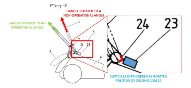
Pet. 35. The annotated version of Figure 10 illustrates handle 1 in operational and non-operational positions, and how cam 24 interacts with actuator 23 based on the handle position.
