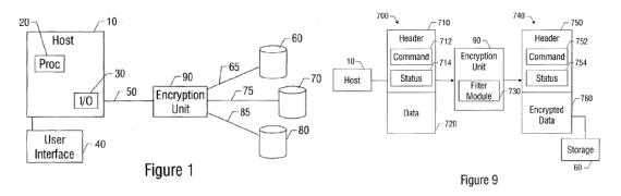
Figure 1 depicts processor-based system 10, which includes subsystem 30 in communication with serial channel or bus 50. Ex. 1002 ¶ 21. Sullivan
